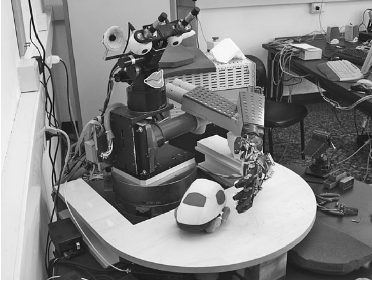
FIGURE 1.7 BABYBOT learns about object properties and affordances by poking and shoving. (From Metta and Fitzpatrick 2003, by permission)
