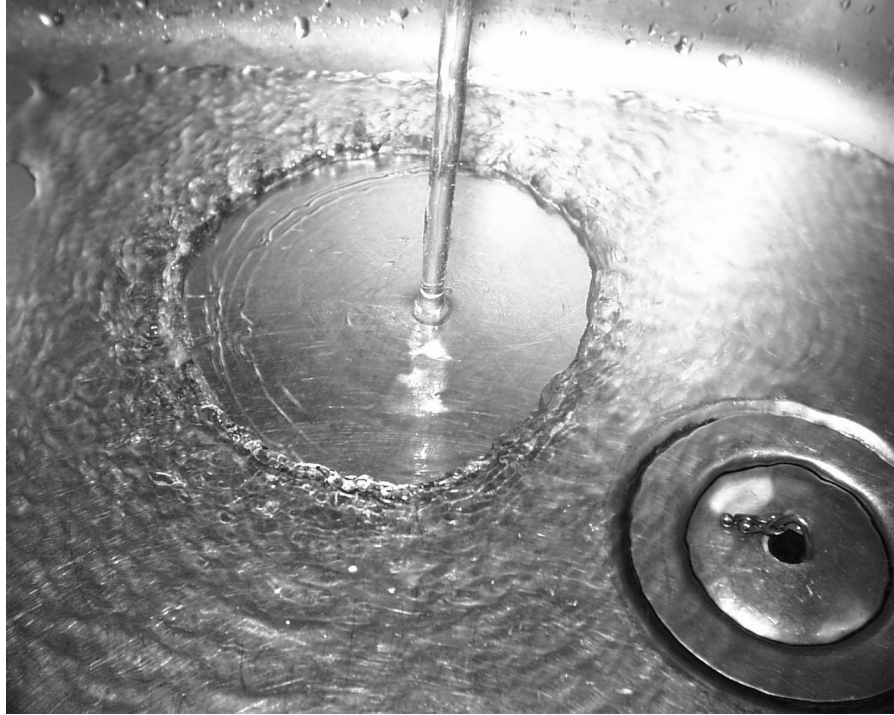
Figure 25.2. Hydraulic jump in the kitchen sink. Photograph by Philippe Belleudy, Université Joseph Fourier, reproduced with permission.
