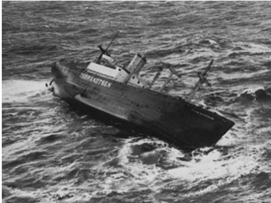
Figure 5.1. The Flying Enterprise (1952). A body can float stably in many orientations, depending on the position of its centre of gravity. In this case the list to port was caused by a shift in the load which moved the centre of gravity to the port side. The ship and its lonely captain Carlsen became famous because he stayed on board during the storm that eventually sent it to the bottom. Photograph courtesy Politiken , Denmark, reproduced with permission.
