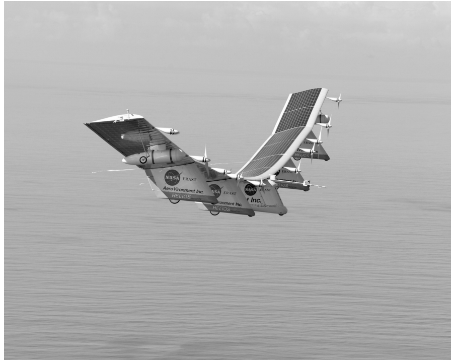
Figure 29.1. NASA's Helios prototype electrically powered flying wing. Image Credit: NASA Dryden flight research center, photo by Carla Thomas.
