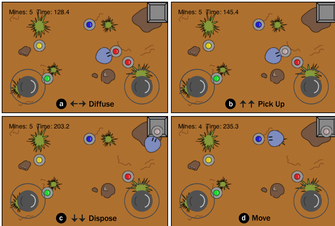
Figure 4.22: In this mine disposal game, the user moves a robot using two joysticks. The left joystick controls movement and the right joystick controls orientation. Two-handed marking menus invoke commands as shown in the four screenshots and can be executed anywhere on the screen.
